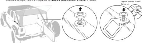
Step 2 Snap the clips onto the Tie-down D-rings with the GPCA cover logo side up.
